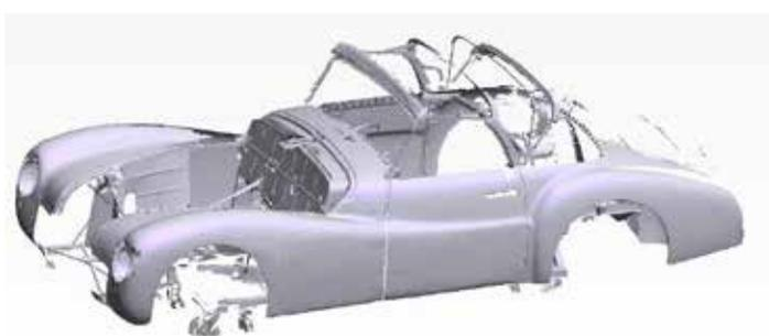
Raw laser scan image of the 1943 Alfa Romeo 6C2500 (photo courtesy of Cooper Technica Inc.)
