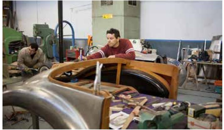
Fitting the trunk panel on the restored rear body section of the 1948 Delahaye at the shop in France (photo courtesy of Cooper Technica Inc.)
