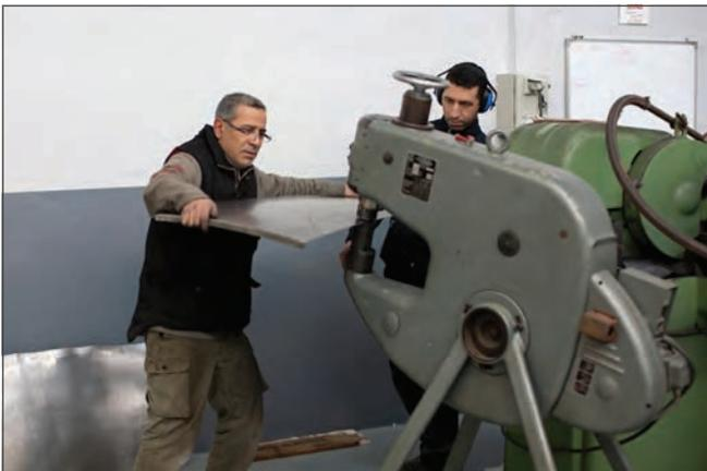
An Eckold Reciprocating machine with shrinking dies removes the stretch from the formed part. Often this is used after the dominant curve has been formed on the Three-Olive machine. (David Cooper)
