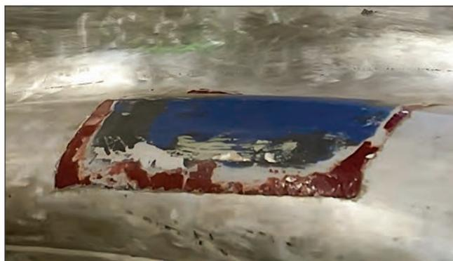
Detail of the original paint layer on 800858 with black paint showing around the edges. The black color, painted by Saoutchik one week after the car was first shown at the *concours*, was applied directly on the blue without primer or resurfacing between the layers. This confirmed the story that the car was quickly repainted for the *Concours d'Élégance* at Enghien. (David Cooper)
