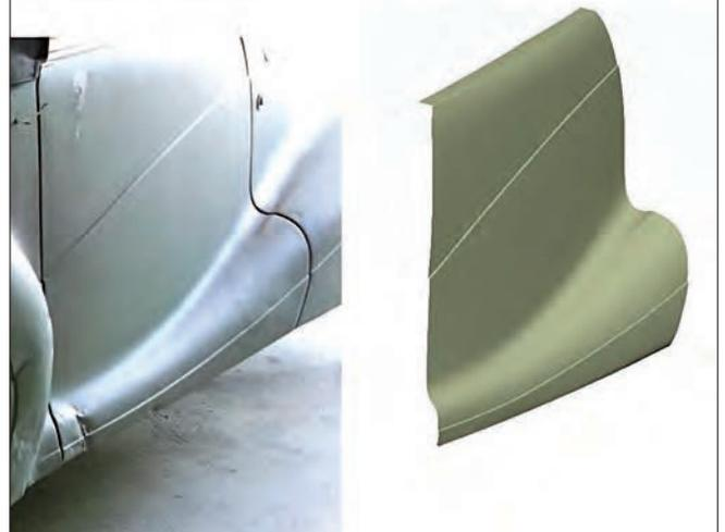
Detail of the digital rendering of the right door of 800858. The original door is shown in the lower left for comparison with the rendering. The rendering forms the basis for fabricating new body maquettes for the sheet metal panels. This allows the original sheet metal door panel to be restored exactly to its correct dimensions. It eliminates distortions introduced in previous repairs. (David Cooper)
