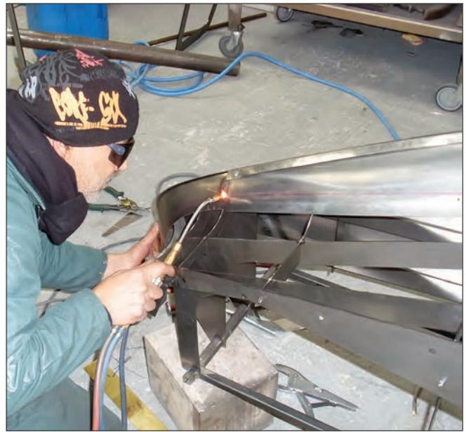
Butt-welding two panels together on a fender by hand using a gas or oxygen-acetylene torch and minimal heat. *(David Cooper)*
