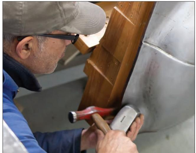
Installing the rear body sheet metal of 800858 around the wood skeleton at the door panel. The sheet metal is wrapped around a steel edge screwed to the wood door jamb support. *(David Cooper)*
