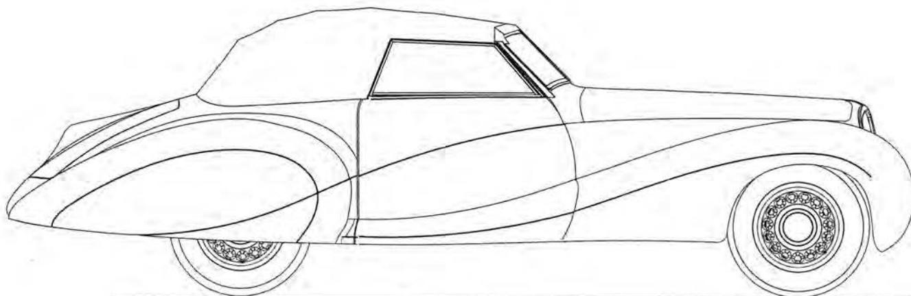
Line drawing by Cooper Technica, Inc. of 800858 in the style of Saoutchik. This drawing was based on a laser scan and reflects accurate proportions and dimensions of the car. (David Cooper)
