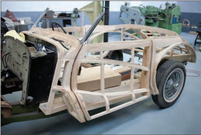
The wood skeleton of 800858 restored exactly as original based on the patterns made from the laser scanned original wood skeleton. The new wood has the same structural integrity as the original. The precision and accuracy of this technique allows the original sheet metal to be preserved and installed on the new wood. *(David Cooper)*
