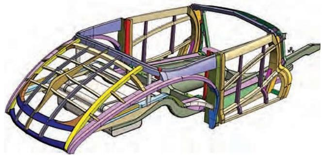
Digital rendering of the wood skeleton for 800858 based on the laser scan of the original wood. This rendering was the first step in creating patterns of each individual wood component so that the wood skeleton could be restored properly. (David Cooper)
