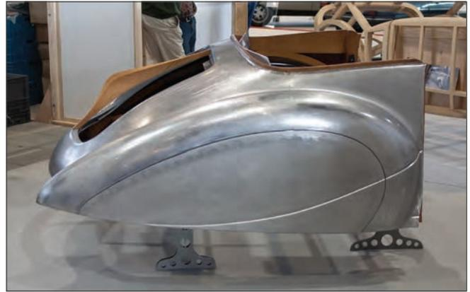
Rear body of 800858. Note the sweep of the curve across the rear wheel skirt. Saoutchik accentuated this curve by swaging the body panel below the curve. He then installed a chrome panel over this embossed section, not shown here. (David Cooper)
