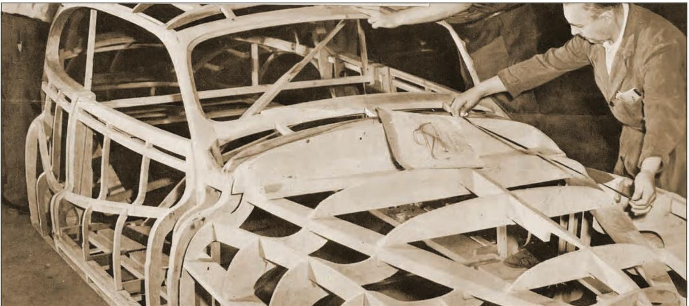
Saoutchik used wood body *maquettes* to fit the sheet metal panels. Here a worker is checking the dimensions. (*France Magazine, Peter Larsen*)
