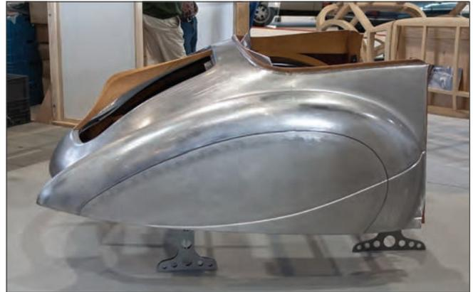
Rear body of 800858. Note the sweep of the curve across the rear wheel skirt. Saoutchik accentuated this curve by swaging the body panel below the curve. He then installed a chrome panel over this embossed section, not shown here. (David Cooper)
