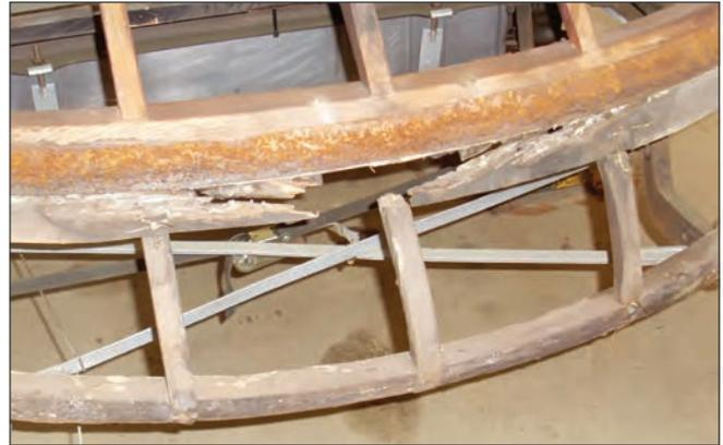
Detail of the damage sustained by the original wood in 800858. The wood supporting the trunk has cracked and rotted. This wood cannot be repaired safely or effectively by splicing and impregnating the wood with resin. (David Cooper)
