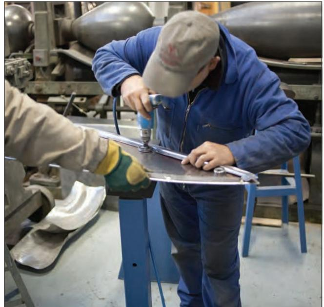
Planishing used to seat the inner structural brace against the sheet metal skin on the inside of the rear wheel skirt. (David Cooper)
