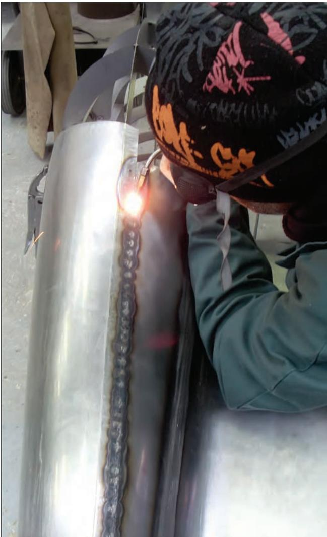
Butt-welding two panels together on a fender by hand using a gas or oxygen-acetylene torch. Note the narrow band of coloration change showing the limited heat used in this type of welding. (David Cooper)
