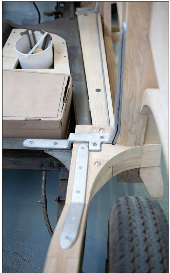
Saoutchik used forged steel body braces to mount the wood skeleton to the chassis. On 800858 he used extra forged steel bracing because he designed large door openings for ease of ingress and egress. (David Cooper)
