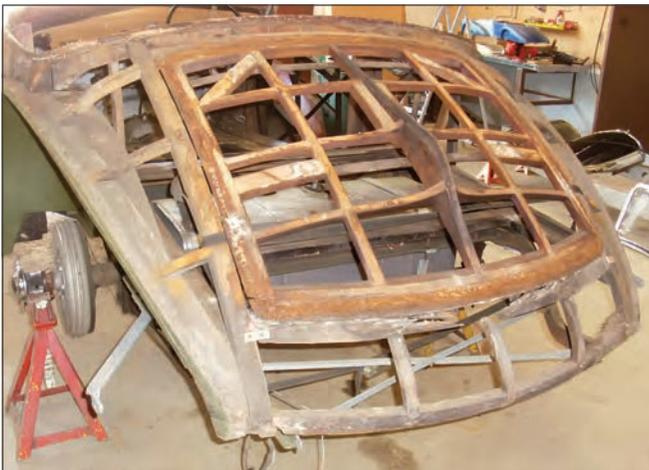
Detail of the trunk area of 800858. Note the damage to the wood below the trunk cover. (David Cooper)
