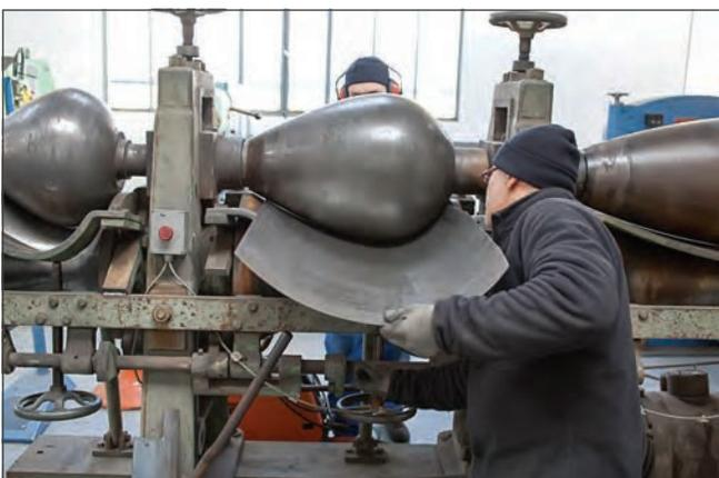
Detail of the part being shaped by the center roller set of the Three-Olive machine. (David Cooper)
