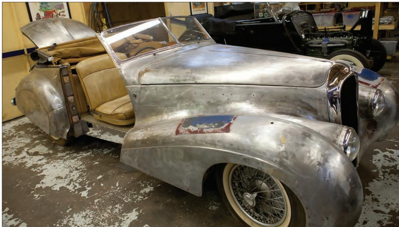
Eleven layers of paint from the body shell of 800858 were chemically hand stripped layer by layer to reveal the original sheet metal. In one area the original dark blue color paint color was left for reference. (David Cooper)
