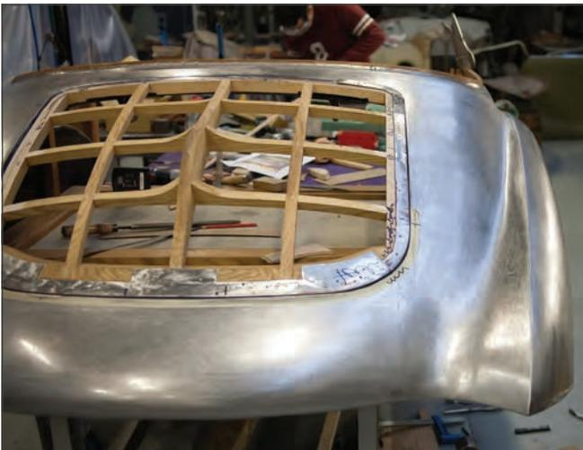
The original rear sheet metal reinstalled on the body of 800858. Over 85% of the original sheet metal could be preserved and reinstalled using this technique. *(David Cooper)*
