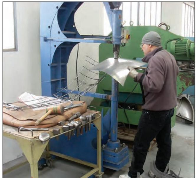
A power hammer is used to form gentle curves in sheet metal parts. (David Cooper)
