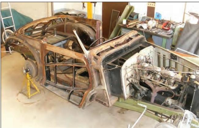
Once the body sheet metal was removed from 800858, the original wood skeleton was exposed for inspection and repair. It had deteriorated badly. (David Cooper)
