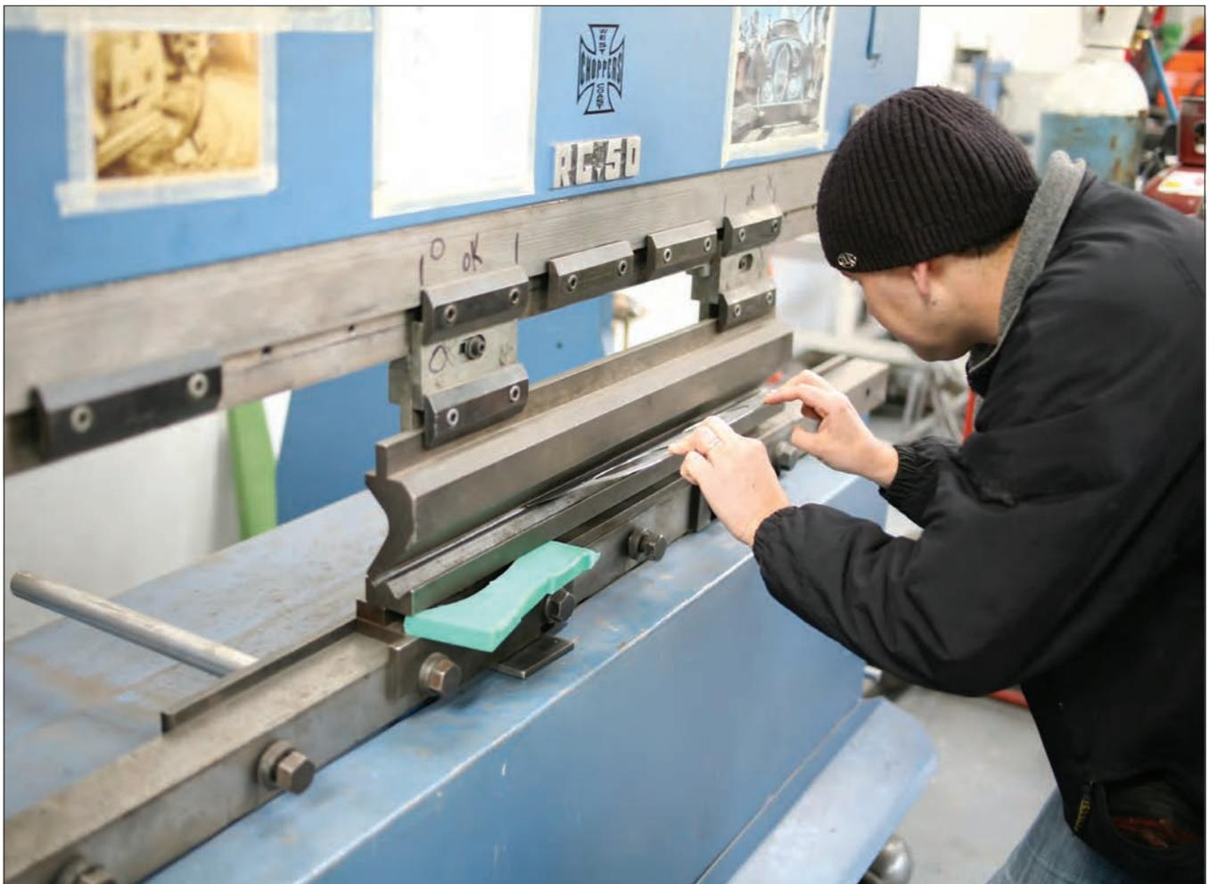
A hydraulic brake is used to bend sheet metal or form it along straight lines. Custom tools are made by the metal shaper for different effects. Coachbuilders formed hood hinges on brakes with special tools. *(David Cooper)*
