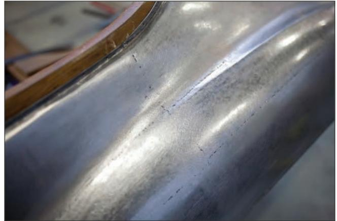
Detail of the rear fender of 800858 showing Saoutchik's original butt-welds on the fender panel. Saving the evidence of Saoutchik's original construction was the purpose of chemically hand-stripping the paint from the sheet metal. The multiple complex curves created by Saoutchik for this design required small sheet metal parts to be formed and welded to make up the fender shape. *(David Cooper)*
