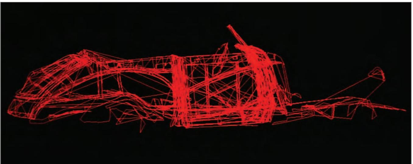
Laser scan of the original wood skeleton of 800858. This scan provided an accurate three-dimensional portrait of the wood skeleton and was used to design patterns for restoring the wood skeleton. *(David Cooper)*
